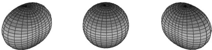
Fig. 2. Geometry of the l = 2, m = 2 oscillation mode.
